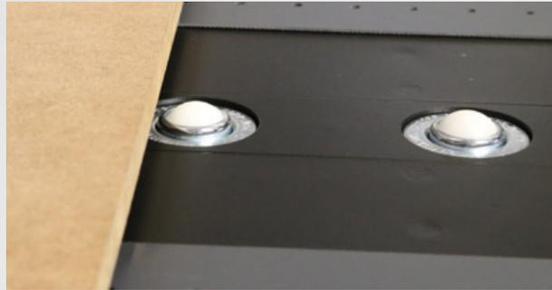
For heavy or large boards, there is a special setting of the automatic board feeder with **ball rollers** that give extra support.
